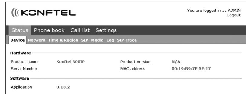
The Device tab shows phone information including serial number, network port and current software version.
