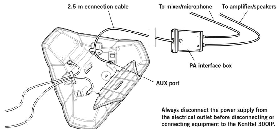
⇒ Connect the PA-box to the AUX port on Konftel 300IP with the included cable.
